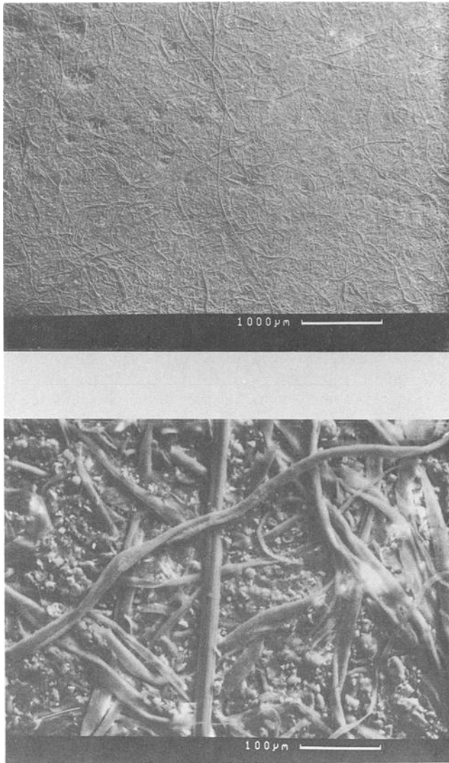
FIG. 3—The coverage of the double-side adhesive by various particles after sampling of a laboratory coat.
